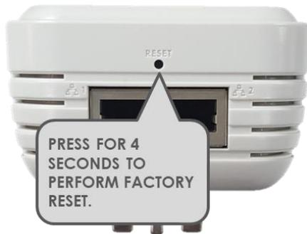
It is highly recommended to perform a factory reset to ensure that all new updates are successfully applied. To do this, simply press the Reset button of your HL129EW for 4 seconds.
