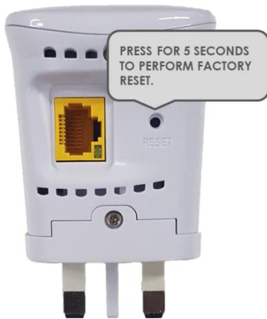
**It is highly recommended to perform a factory reset to ensure that all new updates are successfully applied. To do this, simply press the Reset button of your WL580E for 5 seconds.**
